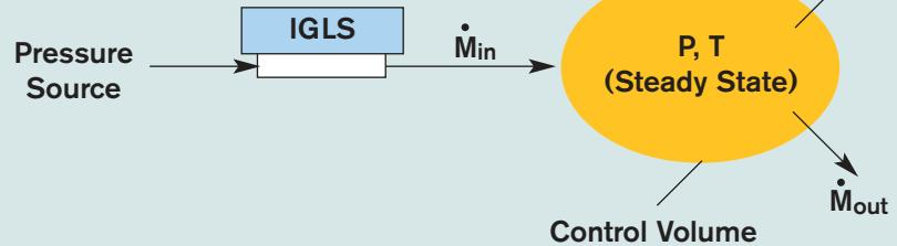
$$\dot{M}_{in} = \dot{M}_{out} \text{ @ steady state}$$
