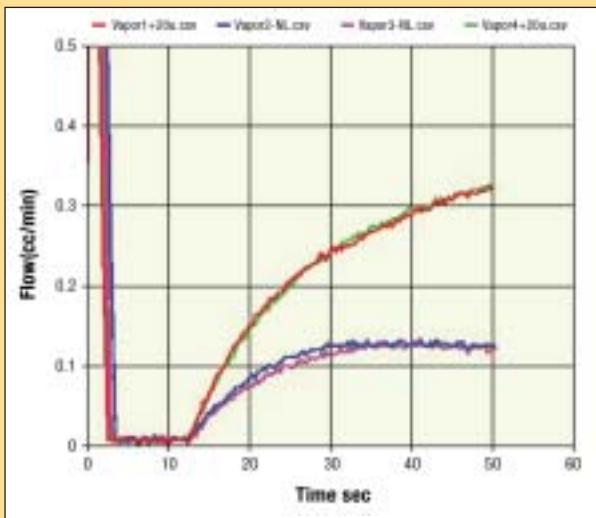
The following example demonstrates the concept of setting up a production leak test system for a product with an Equivalent Channel (EC) specification. The blue and pink lines demonstrate an accepted part. The red and green lines demonstrate a repeat test of the same part with an EC attached to the part inlet. Note the significant increase of leak flow rate because of the attachment of the EC.
