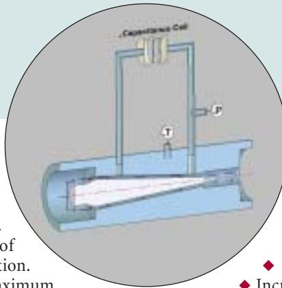
This figure demonstrates the mass flow under air pressure and mass extraction under air vacuum. IGLS/IMFS are micro-flow sensors. A cross section is shown. Source: ATC Inc.
