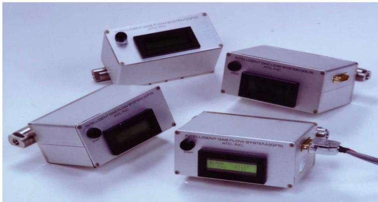
Together with built-in pressure and temperature sensors, accelerated laminar flow technology is the basis of a new type of leak detector called an intelligent gas leak sensor
