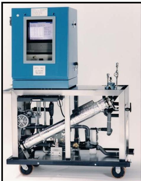
**Liquid Flow & Density Calibration System**
